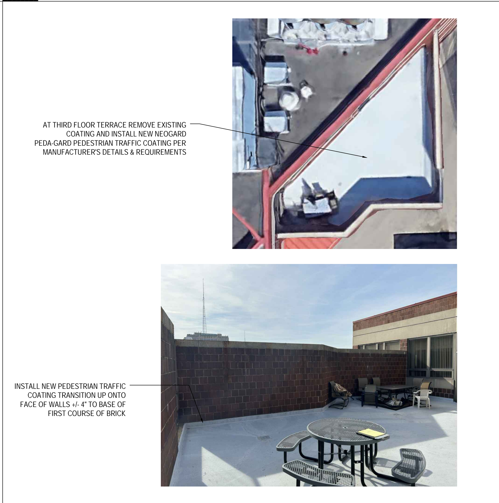
18 D3 TERRACE WATERPROOFING REPLACEMENT DETAIL
