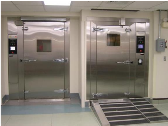
Example of a Cabinet & Rack Washer
