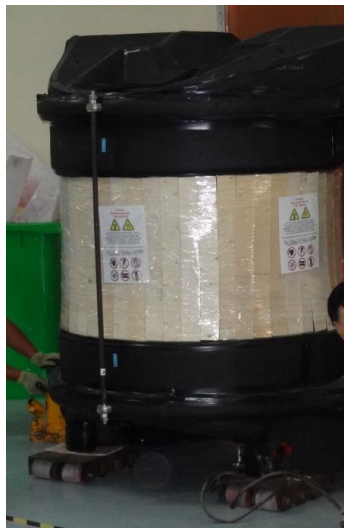
Figure 6: Transportation Protection Bar and Wooden Protective Boards
