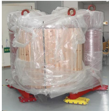
Figure 9: Lifting Eye-Bolts Fixed on Magnet
