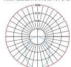
$\label{eq:maximum Candela} {\sf Maximum Candela} = {\sf 2966 \ Located \ At \ Horizontal \ Angle} = 0, {\sf Vertical \ Angle} = 0$
