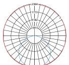
Maximum Candela = 2364 Located At Horizontal Angle = 15, Vertical Angle = 5
