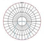
Max Candela = 3899 Located At Horizontal Angle = 0, Vertical Angle = 0
