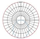
Max Candela = 8407 Located At Horizontal Angle = 0, Vertical Angle = 5
