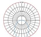
Maximum Candela = 4136 Located At Horizontal Angle = 0, Vertical Angle = 0
